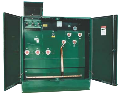
1500KVA Dead Front Radial Feed 3 phase Pad-Mounted 24.9kVGY/14.4 kV - 600Y/347V
