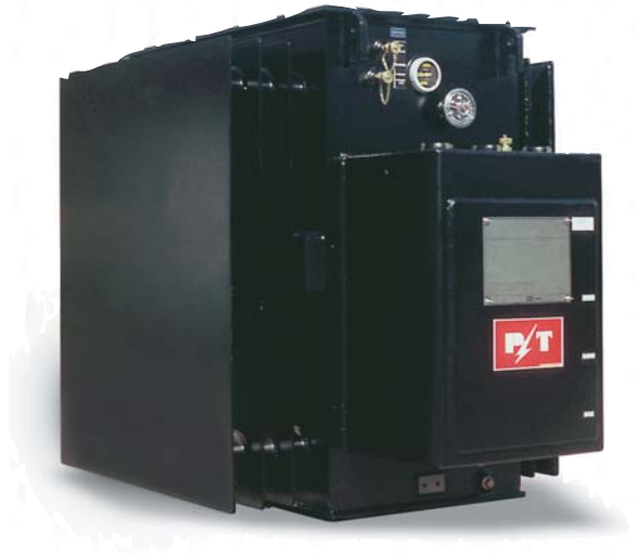
750 kVA 12kV \Delta -480Y/277V Network Transformer
