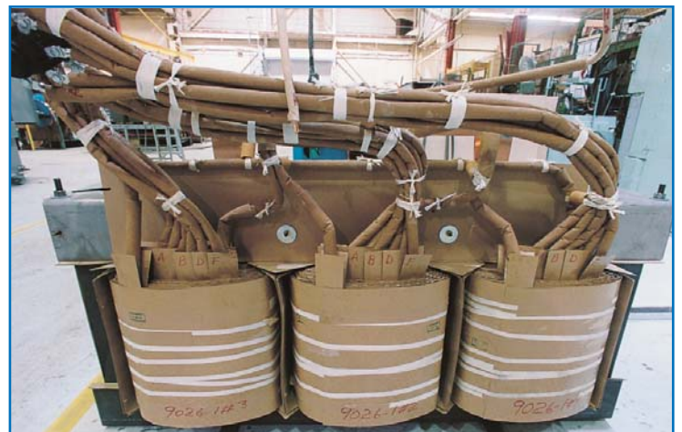
Core & coil assembly
